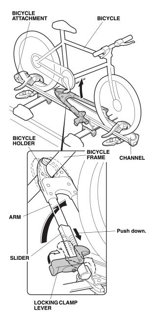
11. Push up the locking clamp lever to secure the bicycle holder.
