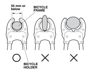
10. Position the bicycle in the channel. Lift up the arm, then clamp the bicycle's frame in the bicycle holder by pushing down the slider.
